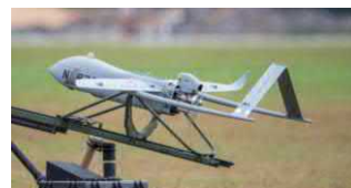
36kg, >10h, 140km, up to 400km with ground relays EO/IR, radar Launcher & net
