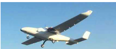
180kg, >10h, 500km(SATCOM) EO/IR, Mar. radar, Still camera, radar detector, phone detector
